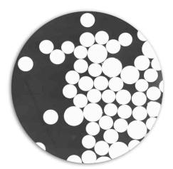
This is a transmission electron microscopy (TEM) photograph of a mixture of our 8070 and 8100 silica particles.
